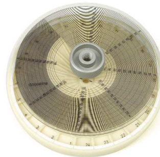
24 place rotor for capillary Microhematocrit tubes. Hematocrit Reader incorporated into the cover
