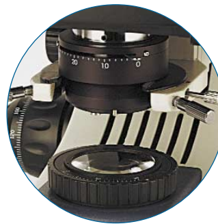
Close-up of graduated Iris diaphragm, graduated Koehler Illuminator diaphragm and graduated fine focus control
